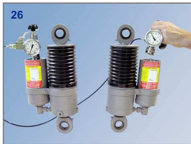
Next, open the purge valve handle (**P**) slowly (image 25) to purge inside the ensemble of the gas charge checkers and the hose. The pressure gauges should read 0 bar once this has been accomplished.
