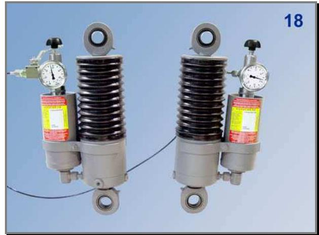
Turn the shaft handles (**G**) (image 17) in both gas charge checkers slowly and clockwise (it is not necessary to make this with both at the same time) until the pointers in both pressure gauges dial the accumulators gas charge pressure (when the pointers stop moving on the scale).
