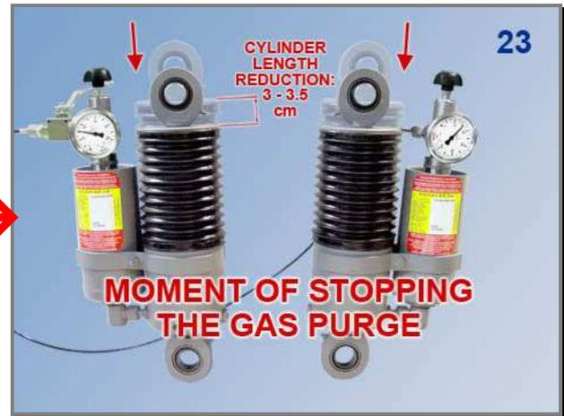
Now turn both checker shaft handles (**G**) fully counter-clockwise (image 24) in order to close the exit of the gas from the accumulators (They can feel more difficult to tighten now than when tightened before, as now the pressure of the gas inside the gas charge checkers ensemble is opposing the turning movement).
