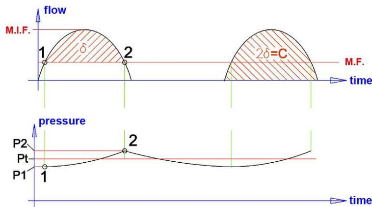
**Figure 5.** Pressure evolution in 1 piston pump complete cycle with the installation of a pulsation dampener.
