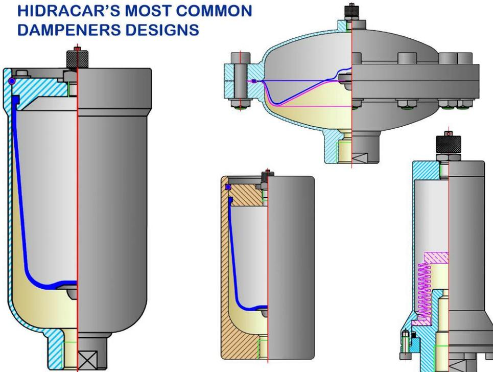
**Figure 1.** HIDRACAR's most common dampeners designs. (Bladder, Bellows and membrane types)
